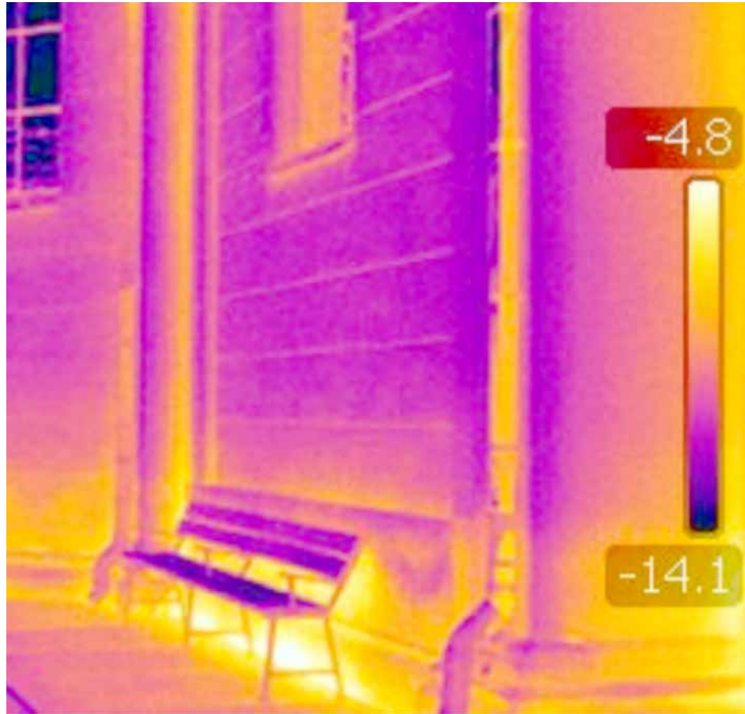
(Left) A thermal image showing thermal bridges on an exterior wall. (Above). Heat loss around an exterior garage door at St. Luke's Camden East. Photos-EF Turcanu, Ian Kilborn.
