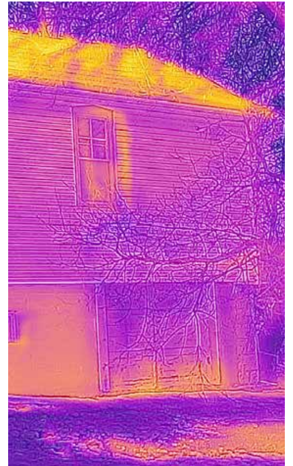
(Left) A thermal image showing thermal bridges on an exterior wall. (Above). Heat loss around an exterior garage door at St. Luke's Camden East. Photos-EF Turcanu, Ian Kilborn.
